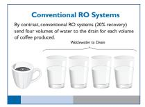
A conventional RO system can require five volumes of water to produce one volume of water that can be dispensed. The remaining four volumes are discharged to drain. The MRS-600HE systems waste only a small fraction of the total volume, thus reversing the ratio of waste-to-product RO water relationship.
